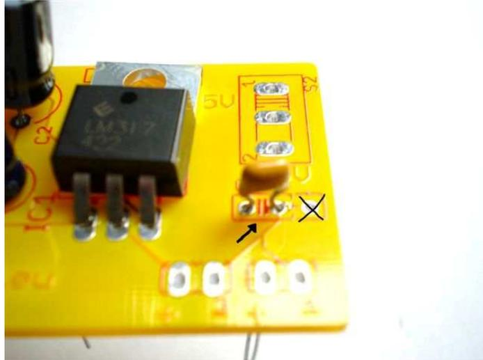
Bend the 4 resistors as shown and place the different values in their right place. R1=240 Ohms, R2 = 390 Ohms and R3 + R4 are both 330 Ohms. Look at the colour codes and at the picture to see how they must be connected.
