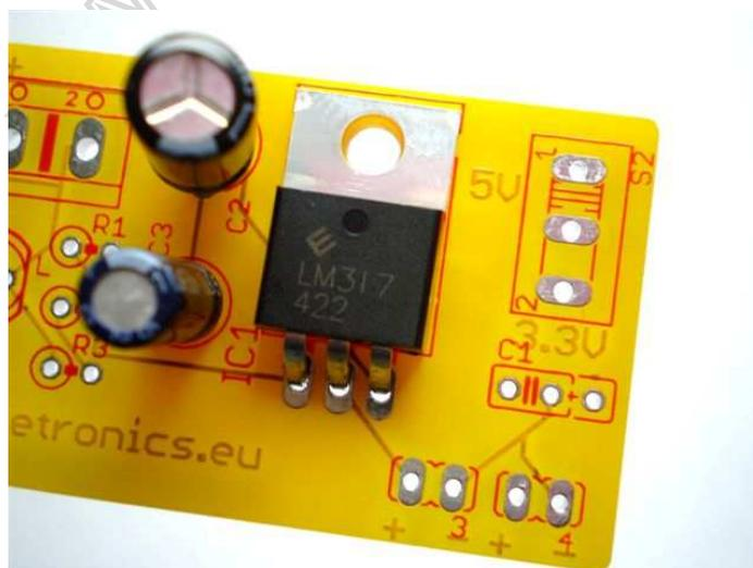
Place the ceramic capacitor in its position. It does not matter how you connect this. You see in the picture that one hole is crossed out. Don't use this hole. Just connect the capacitor exactly as shown in the picture.
