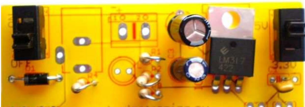
Put the block terminal in place with like shown in the picture.
