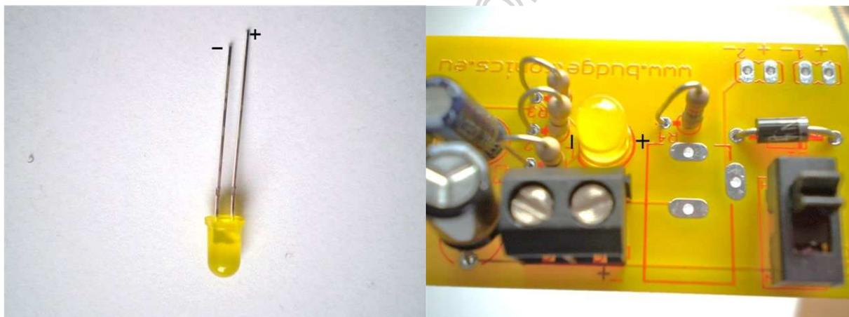
Look closely at the picture how to connect the LED. The LED shows you when the power supply is switched on.
