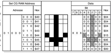
3.) The new defined character can be used as a "normal" ASCII code (0..7); use with "DD RAM Address Set" and "Data Write".
