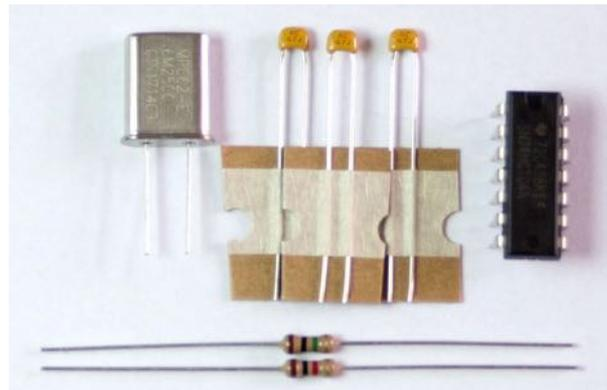
Apart from the chip, all components can be soldered in either orientation. See chapter 4 for more information about how to bend the pins of the IC to get it to fit into the board. If you solder it the wrong way around, cut the pins and remove them one by one, and request a new IC from us. In our experience, trying to get out the IC in one piece often results in damage to the board. This is true for all the IC's you are about to solder.
