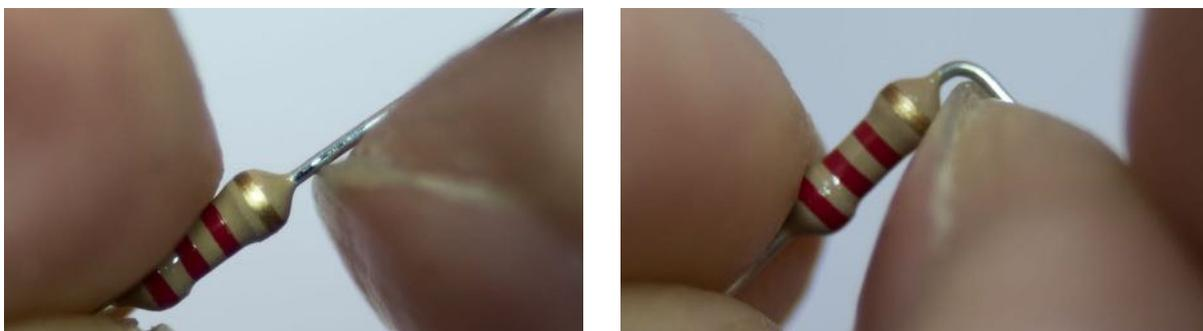
Now you can place the resistor (or other component) into the PCB (on the printed side). On the bottom of the PCB, the pins stick out. Resistors and some other components sit on the PCB. If you bent the pins correctly, the resistor should be in place. You can push the component down if it "almost" fits, the pins will then bend the last bit to match the holes.
