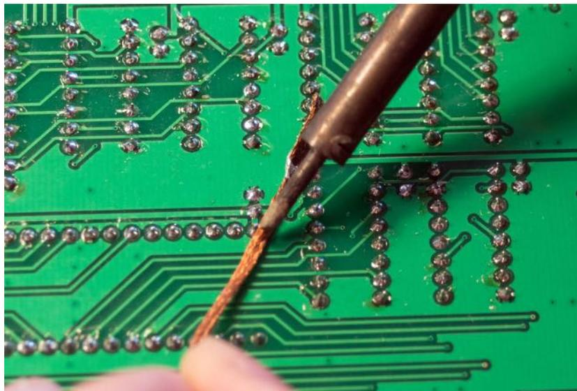
*Using desoldering wick*
