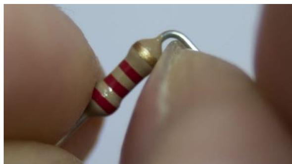
Now you can place the resistor (or other component) into the PCB (on the printed side). On the bottom of the PCB, the pins stick out. Resistors and some other components sit on the PCB. If you bent the pins correctly, the resistor should be in place. You can push the component down if it "almost" fits, the pins will then bend the last bit to match the holes.
