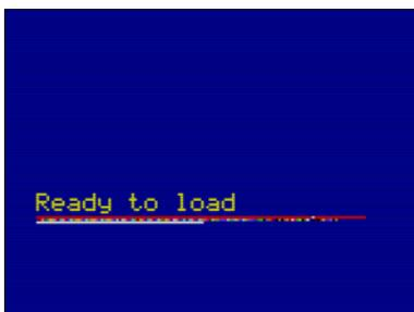
The loader listens to data packets on the controller port and stores them in memory. You can hook up an external device to the controller port and send commands or complete new programs into the `gigatron` this way and run them. The PS/2 adapter can send BASIC using the loader. When in the loader, press Control-F1 to activate this. Loading BASIC this way is only needed for older ROMs, that do not contain BASIC. In your system, you can just run BASIC from the menu.
