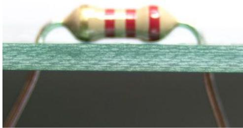
Now you can start to solder. Make sure the soldering iron is up to temperature and be sure not to touch the metal half as it gets hot. Hold it against the PCB like a pen, just where the pin sticks through and heat it up for a second. Then, use your other hand to add solder, that will start to melt. Add the solder at the joint of the pin and the PCB, do not put it on the soldering iron. Remove the solder and remove the soldering iron.
