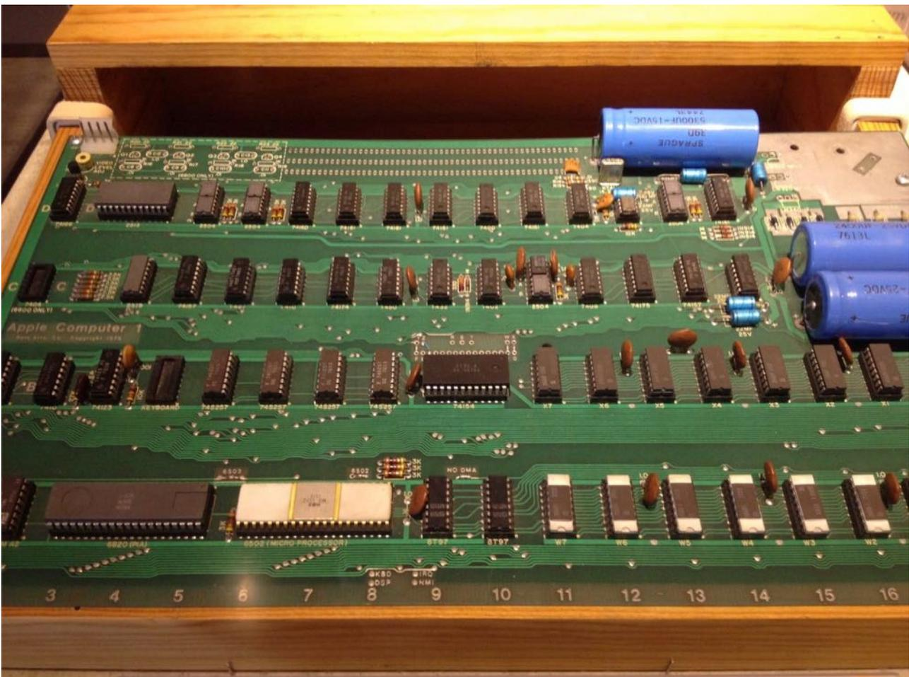
The large white chip is a 6502 CPU, running at 1MHz.
