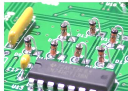
padded hole. In short: the diodes are on the left with the black ring on top, the wires are on the right.
