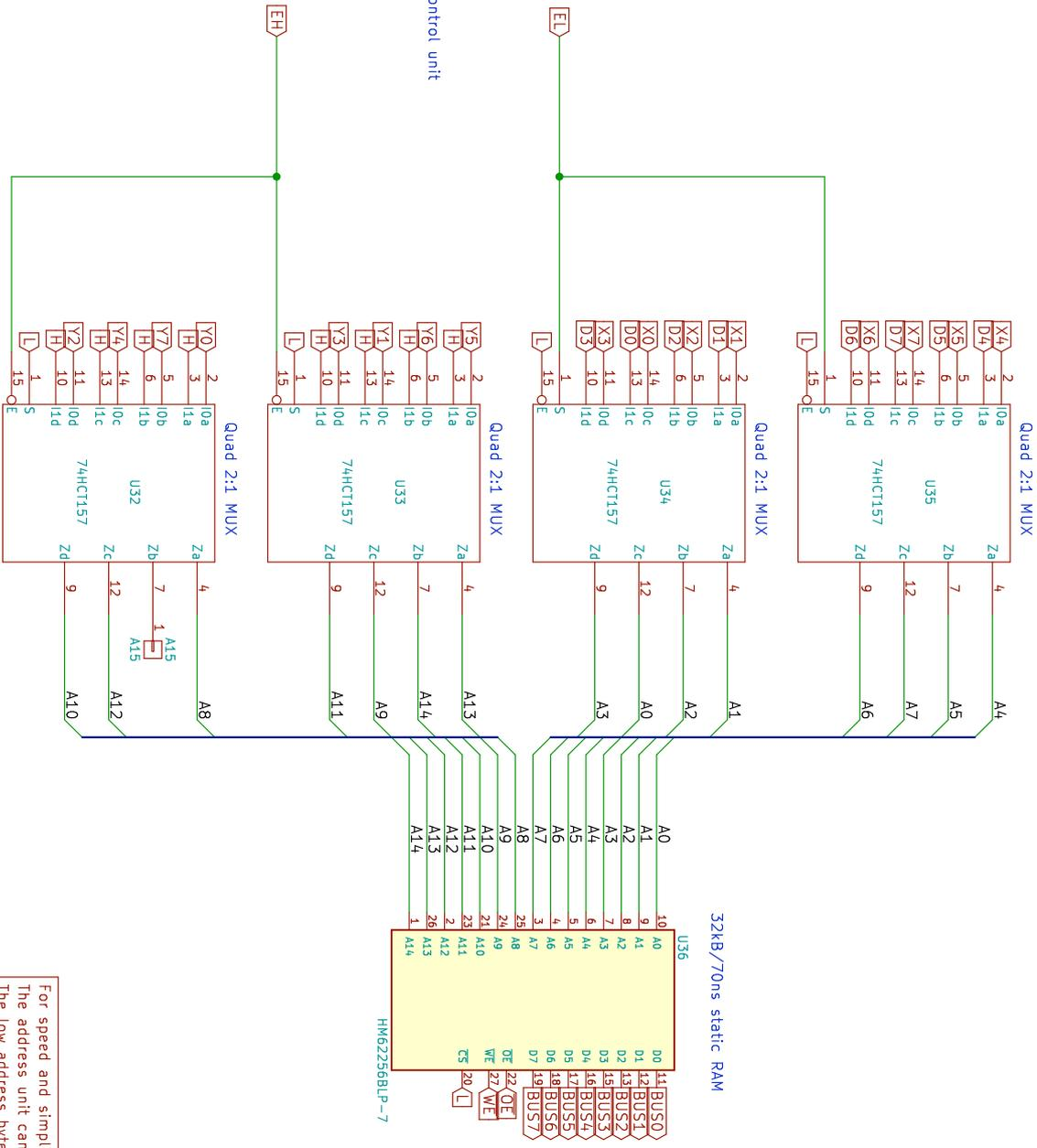
The 6.25 MHz system has a clock period of 160 ns. In each clock cycle 1 RAM access and 1 ALU operation can be done sequentially. Therefore the computer needs an SRAM speed of 70ns for reliable operation. In the kit 55ns SRAM is included for additional headroom.
