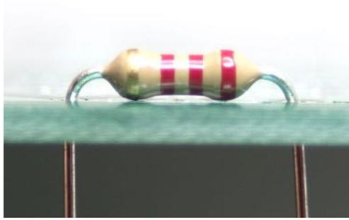
Slightly bend the pins to the side, so the resistor will not fall out when you flip the PCB around:
