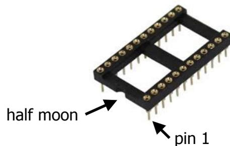
An IC socket also has a half-moon shape cut out, which marks the side where pin 1 can be found.
