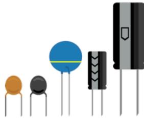
In the picture above, we see ceramic capacitors on the left. These are normally small, in the pF to nF range. They have no polarity, meaning they can be used either way around. The electrolytic capacitors have higher values, in the  $\mu\text{F}$  range. They are polarized, meaning it matters in what orientation you solder them in the PCB. The white band, in many cases filled with minus signs, points to the negative side. On the PCB, we have marked the orientation of these capacitors.
