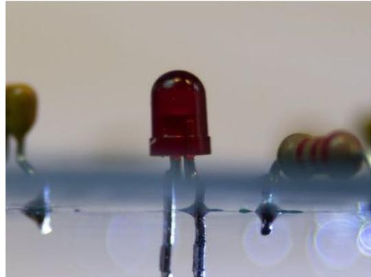
Next, apply heat from the soldering iron while, again **gently**, pushing the LED in the correct position. When you are satisfied, solder the other lead and re-heat the first one to make sure both leads are soldered well.
