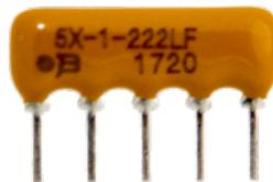
There is always a marking (dot, stripe, ...) at the pin that is common for all resistors. This means that it matters in what orientation you solder them in the PCB. "PCB" stands for Printed Circuit Board, the board that holds all the components and interconnects them.
