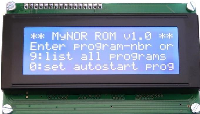
BUT to see this screen you have to adjust the LCD contrast. This is done with TR4 at the left side of the LCD extension board.
