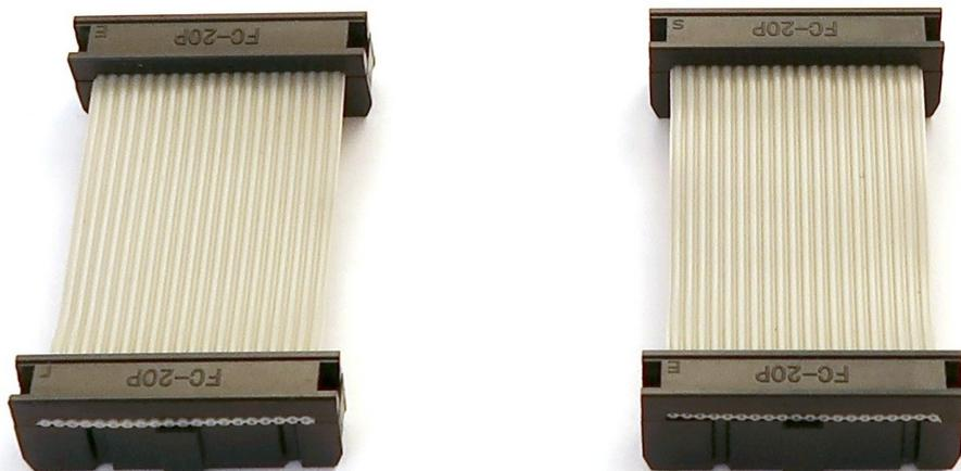
You need to build two jumper cables to connect the LCD extension board to the MyNOR computer board. The following picture shows how the LCD, the LCD extension board and the MyNOR baseboard are assembled together:
