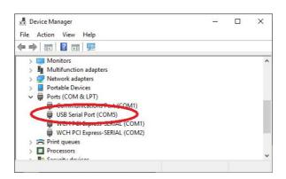
Once this is done you should note the port number created by your computer for the virtual serial connection. In Windows this can be done by starting Device Manager and checking the "Ports (COM & LPT)" entry for a new COM port as shown above.
