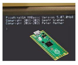
The PicoMiteVGA is a Raspberry Pi Pico running a full featured BASIC interpreter with support for a VGA monitor and a PS2 keyboard for the console input/output.
