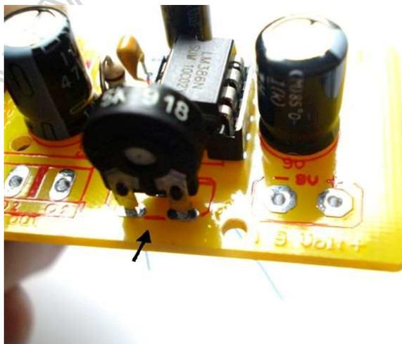
Install the Block terminal as shown on the picture.
