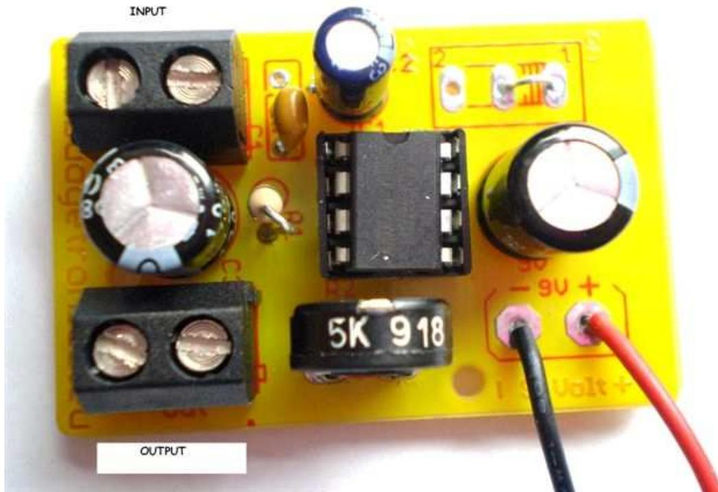
A Budgetronics building kit to make your own mini amp, based on the LM 386 op amp. Handy for amplifying weak signals on a headphone like for instance from a crystal radio. You could also connect a small loudspeaker to it. If you want to amplify a stereo signal you can use two mini amps. One for each channel. Easy connection of output and input signals with block terminals screw connection.
